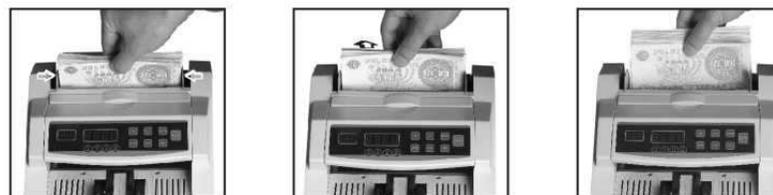
**Note:** The counting mode can be changed between Automatic and Manual. Press the RESTART button for 3 seconds, if the batch display shows YES , the machine is in automatic counting mode;
